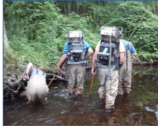
Electrofishing crew using two backpack units along the margin of a small stream.
